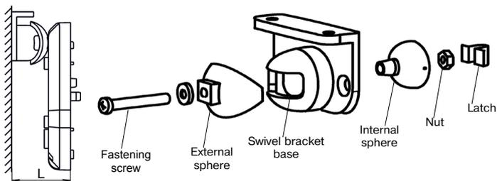
Figure 4 – Swivel bracket fastening and mounting
